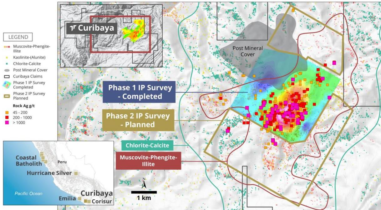
Figure 2: Illustrates the expanded IP program that is planned at the main Curibaya target area due to the extension of the high temperature alteration footprint, consisting of a muscovite-phengite-illite assemblage with associated high-grade silver veins.
